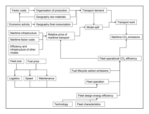
Figure 6-2 – Stylized representation of factors determining maritime emissions
