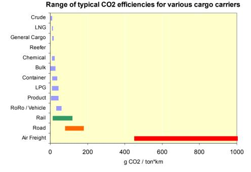
Figure 9-3 - Typical range of ship CO<sub>2</sub> efficiencies compared to rail, road and airfreight
