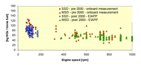
Figure 4-3 – NO<sub>x</sub> emission factors from measurement and from EIAPP certificates
