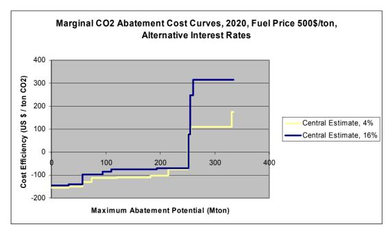
Figure A4-3 – Marginal CO<sub>2</sub> abatement cost curves for a fuel price of US\$500/tonne and alternative interest rates, central estimate only
