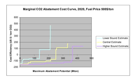
Figure A4-1 – Marginal CO<sub>2</sub> abatement cost curve for 2020, a fuel price of US\$500/tonne and an interest rate of 4%
