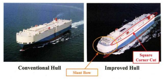
Figure A2-4 – Example of improvements to a superstructure (Universal Shipbuilding)
