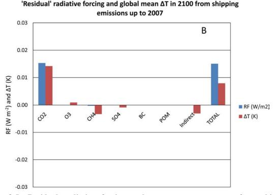
Figure 8-5 – Residual radiative forcing and temperature responses from shipping emissions to 2007 in 2050 (panel A) and 2100 (panel B). The figure does not include the positive RF that could potentially occur from the interaction of BC with snow that has, so far, not been investigated for ships.
