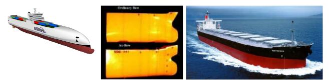
Figure A2-2 – (a) Example of a superslender monohull with outriggers (copyright STX Europe, 2008). (b) Axe-bow design and 172 000 DWT Capesize bulk carrier KOHYOHSAN, built with an axe bow for Mitsui O.S.K. Lines, Ltd in 2001.
