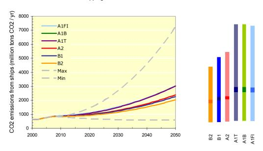
Figure 1-2 – Trajectories of the emissions from international shipping. Columns on the right-hand side indicate the range of results for the scenarios within individual families of scenario.
