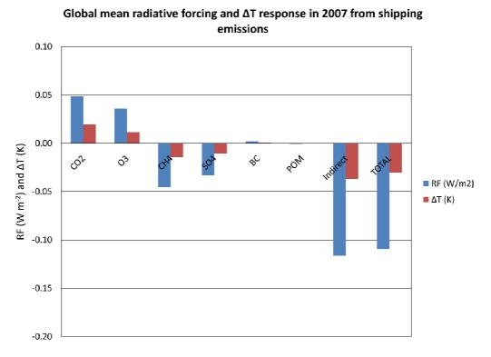
Figure 8-4 – Global mean radiative forcings (W m<sup>-2</sup>) and temperature responses (K) in 2007 from shipping emissions. The figure does not include the positive RF that could possibly occur from the interaction of BC with snow, which has so far not been investigated for ships.
