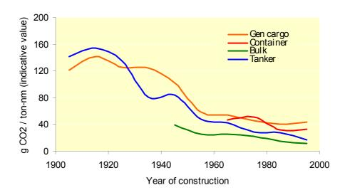
Figure 9-4 – Indicative development in average ship design transport efficiency
