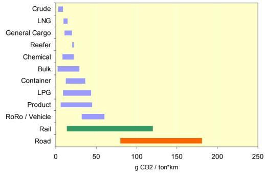
Figure 1-3 – Typical ranges of CO<sub>2</sub> efficiencies of ships compared with rail and road transport
