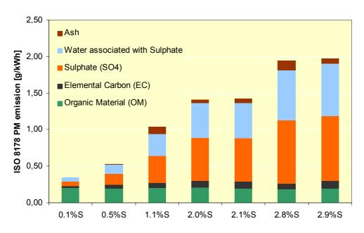
Figure 7-6 – The compositions of particulate matter obtained from different fuel types, Germanischer Lloyd [24]
