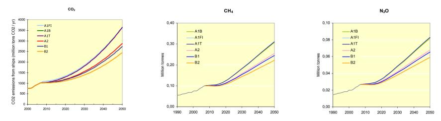
Figure 7-8 – Emission scenario trajectories for GHG emissions – total shipping (exhaust emissions only)
