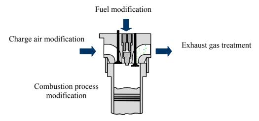
Figure A2-6 – Ways to reduce NO<sub>x</sub> emissions from a marine diesel engine
