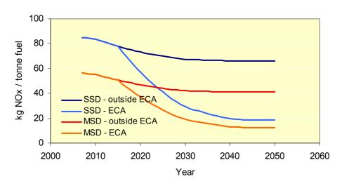
Figure 7-4 – Future NO<sub>x</sub> emission factors (3% fleet growth per year, 30 year vessel life)
