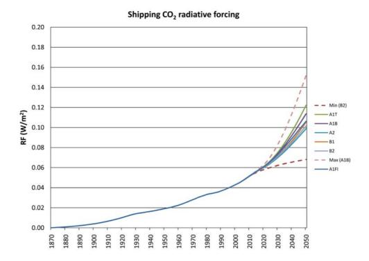
Figure 8-3 – Radiative forcing of CO<sub>2</sub> attributable to shipping from 1870 to 2005, and thereafter, according to a range of scenarios, to 2050
