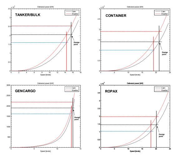
Figure A3-3 – Speed loss (drop) at constant delivered power  $P_{\rm D}$  or at increased delivered power  $P_{\rm D}$ , at constant speed, of the advance of vessels in head weather conditions (irregular waves and wind from the same direction 180°) for four different types of ships, according to MARINTEK's 2008 direct model tests database, with the assumption of Beaufort number BN (Bft) = 6 for Tanker/Bulk, BN (Bft) = 6 for Container, BN (Bft) = 3 for GenCargo, BN (Bft) = 6 for RoPax
