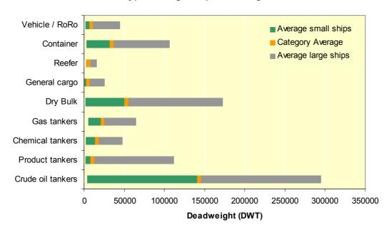
Figure 2-6 – Deadweight of major cargo ship types. High and low end represent average deadweight of the upper and lower ship size categories that were used in the study, not of individual ships, which may be significantly larger or smaller [Lloyd's Register – Fairplay, 2007]
