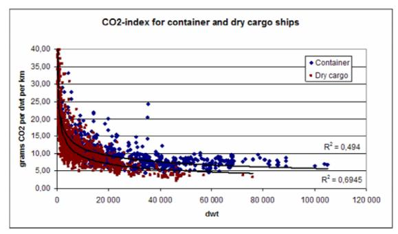
Figure 6-1 – The effect of ship deadweight on CO<sub>2</sub> design index [2]
