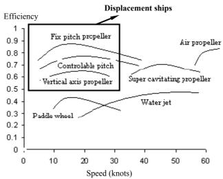
Figure A2-6 – Efficiency of propulsive devices [31]
