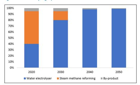
Figure 3.11 Assumed hydrogen production mix
