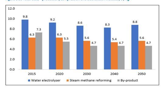
Figure 3.10 Total costs - production, compression and distribution included, € / kg
