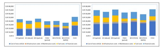
Figure 5.5 Lifetime TCO for all powertrains segment A+B (left) and C (right) in 2030.
