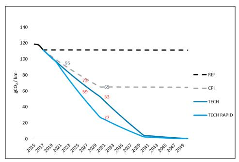
Figure 8.1 Average CO<sub>2</sub> emissions (NEDC) of new cars from 2015-2050
