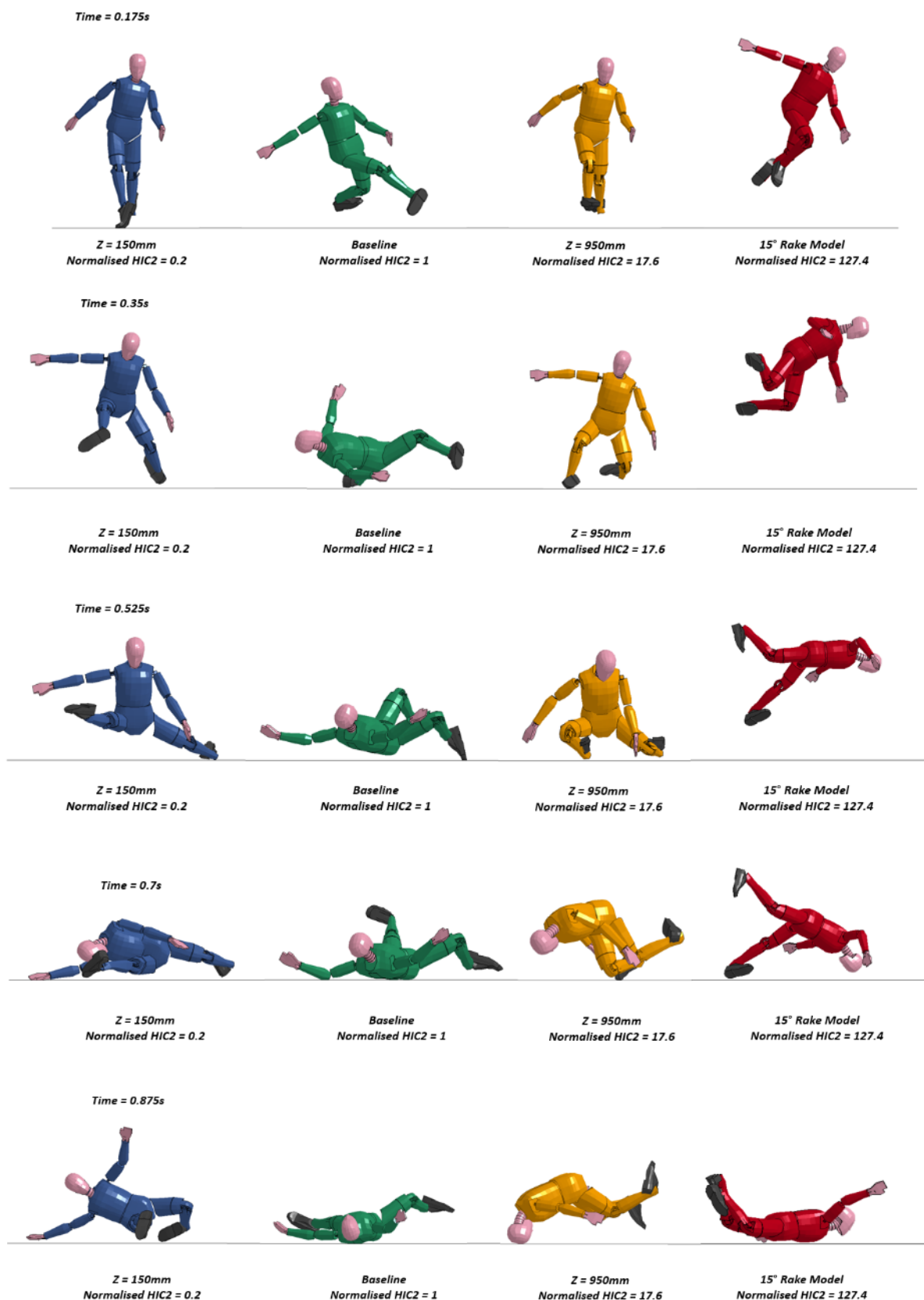
Figure 4: Pedestrian motion and HIC in ground impact for the dual rake cab with a transition height of 150mm, the baseline cab, a dual rake cab with a transition of 950mm and a single rake cab at 15 degrees.
