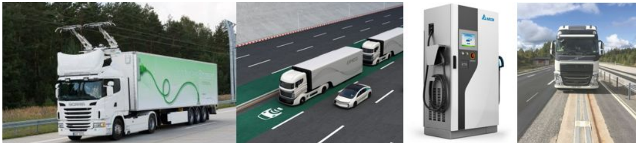
Figure 6: Examples of electric truck charging (from left to right): dynamic via catenary, dynamic via induction, static via plug, dynamic via rail
